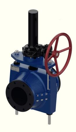
The RHINOFLEX EN-Series is a compact, rugged and robust Pinch Valve. These valves are reliable and maintenance free and are engineered and designed for highly abrasive and aggressive slurry applications. The series has a simple yet trustworthy design, consisting of two pinch bars that open and close the Elastomer
